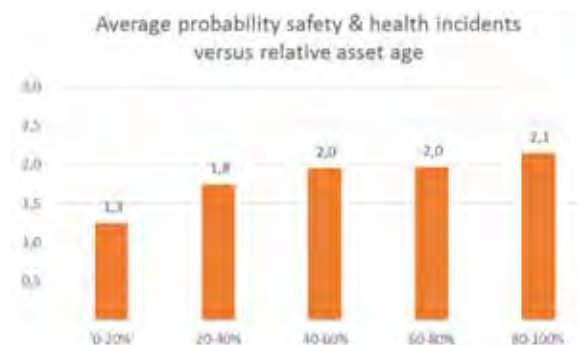
Figure 3.4.3 Relative age of plants and probability of the occurrence of health & safety incidents
